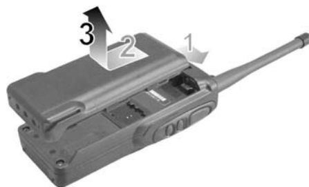
Figure 2.3 – Removing the battery
