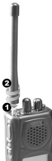
Figure 2.1 – Installing the Antenna
