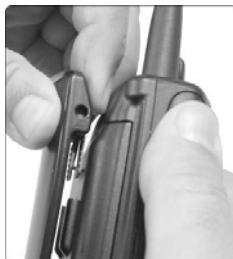
Figure 2.4 – Installing the belt clip
